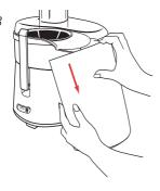
3. Place fingers under the bottom of the twin-locking handles and lift to release – figure 9.
